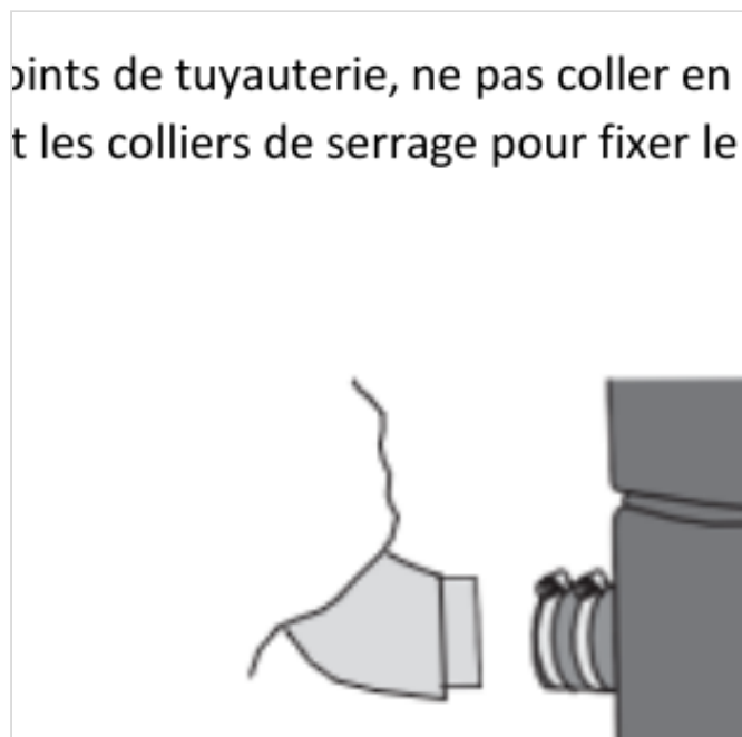
Final fitting : sleeve + clamps, not glued.
