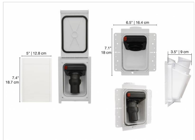
Retractable wall inlet with its rough-in dimensions.
